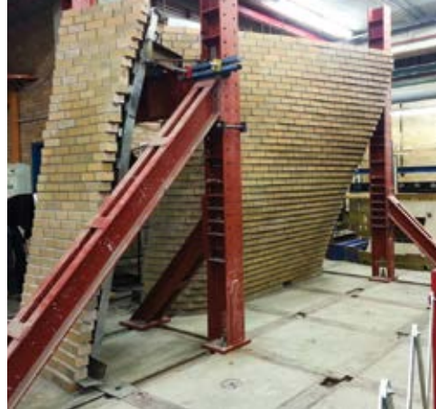
Figure 7. Full-size mockup panels before load testing.
