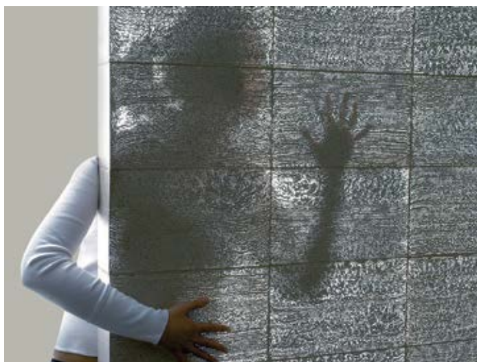
A concrete panel made with Litracon material.
