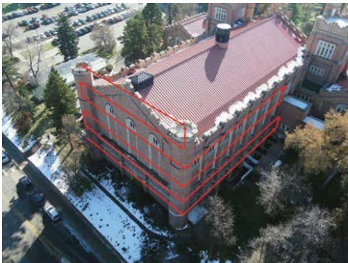
Figure 4. Preprogrammed flight path for façade mapping.
